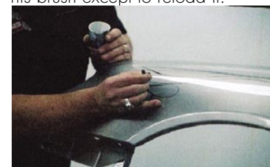
Tex demonstrates striping on a front side quarter panel
